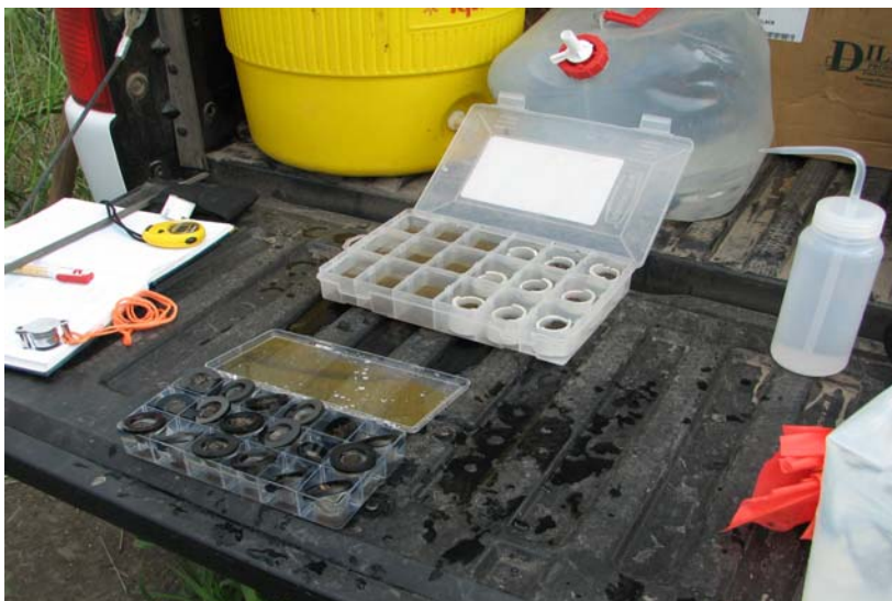
Fig. 2 Method to test water stable aggregates of the surface 1 inch of the soils in each rotation. Sampling procedure was 15 samples per site. See Table 4.
