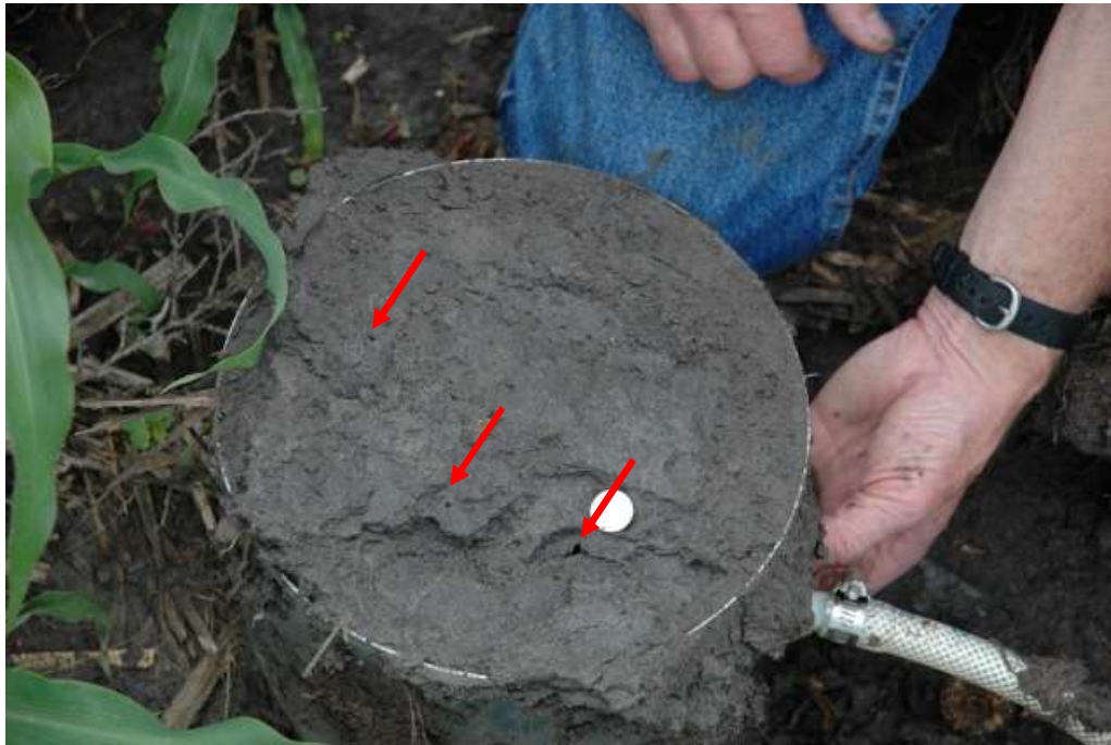
Fig. 2 Ring for infiltration is 9.5 inches in diameter, observing different sizes of soil pores. Dime offers reference of some of the 2 to 5mm pores pointed out by red arrows.
