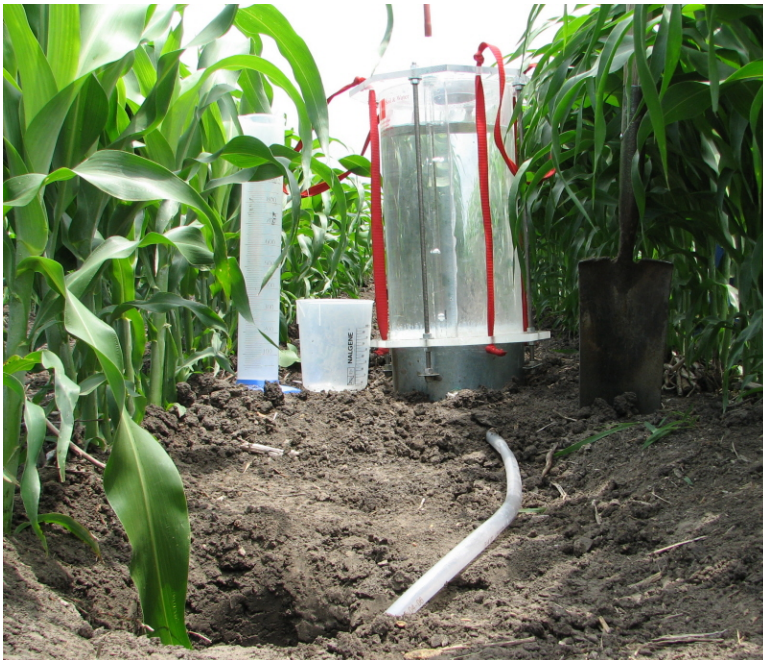
Fig.1 The photo to the left shows the Cornell Sprinkle Infiltrometer in the corn on cotton area of the crop and tillage rotation study on the Stiles Foundation Farm near Thrall, Tx. Photo Courtesy Orthman Mfg.
