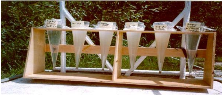
Fig. 1 Image of Imhoff Cones used to determine water quality and sediment loading
