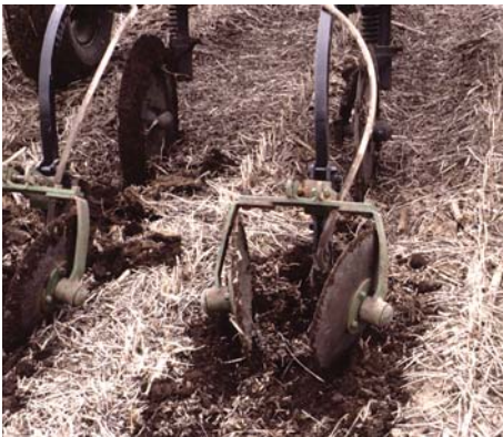
Fig. 5: Strip-tilling with an anhydrous ammonia knife and covering discs.
