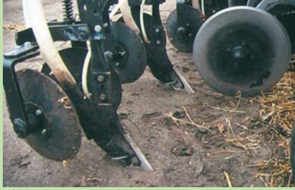
Fig. 1: Coulter, fertilizer injection knives, and covering disks on strip-tillager.
